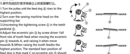
1. Turn the pulley until the feed dog ① rises to the highest position.
