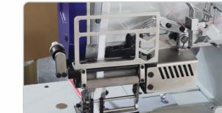
Step motor control belt feed system
